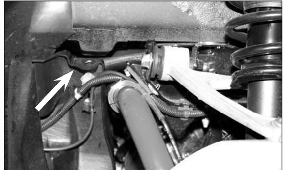
Remove the plastic under tray retaining bolts.
